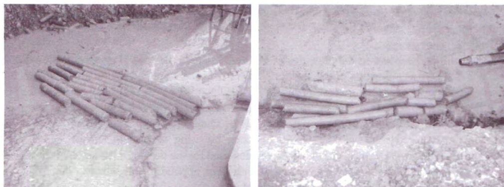
Figure 23. Clay samples from borehole operations.
