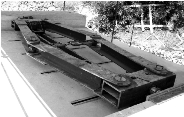
Figure 10. Sudden release device – Prototype. Figure 11. Fuse: calibrated HS steel rod.
