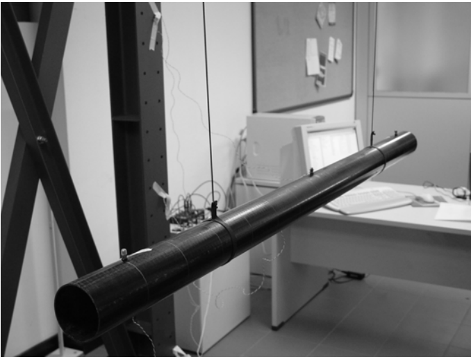
Figure 3. Test object, grid of measurement points, suspension system and M353B17 PCB piezoelectric accelerometers located on a straight line.
